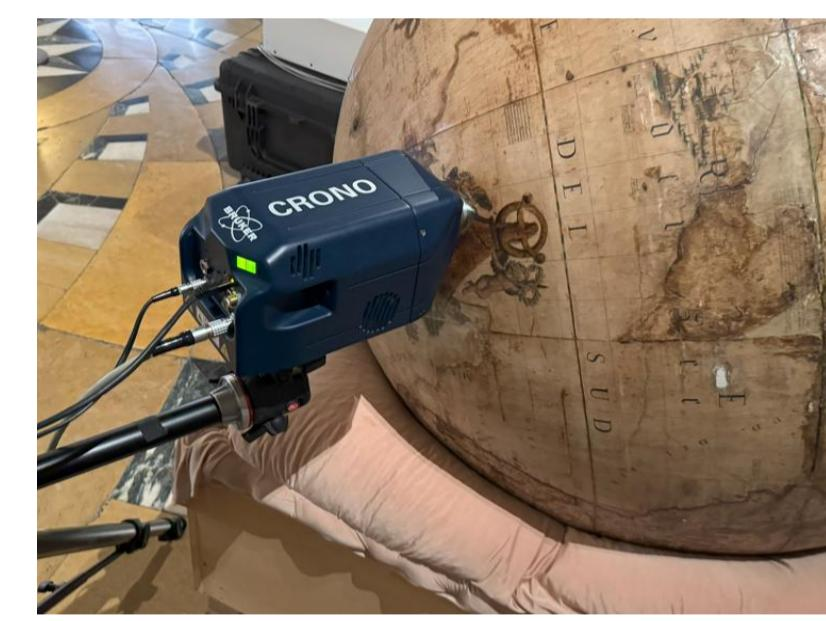
**XRF spectroscopy:** *Crono* (Bruker) XRF spectrometer
