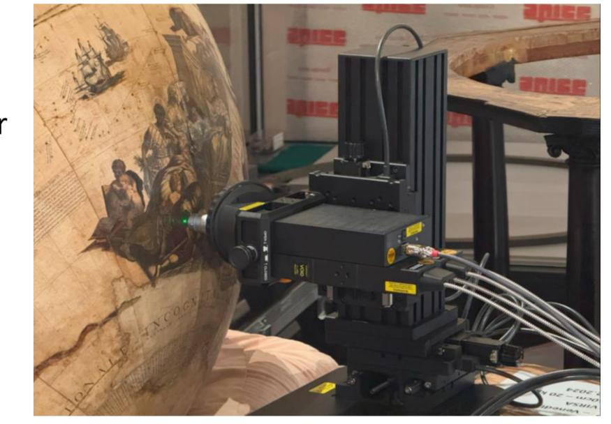
**Raman spectroscopy:** *Virsa* (Renishaw) Raman spectrometer
